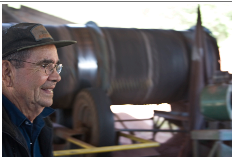
Ray and the brick tumbler he had built to turn bricks with flaws into old looking bricks for restoration projects and antique style.
